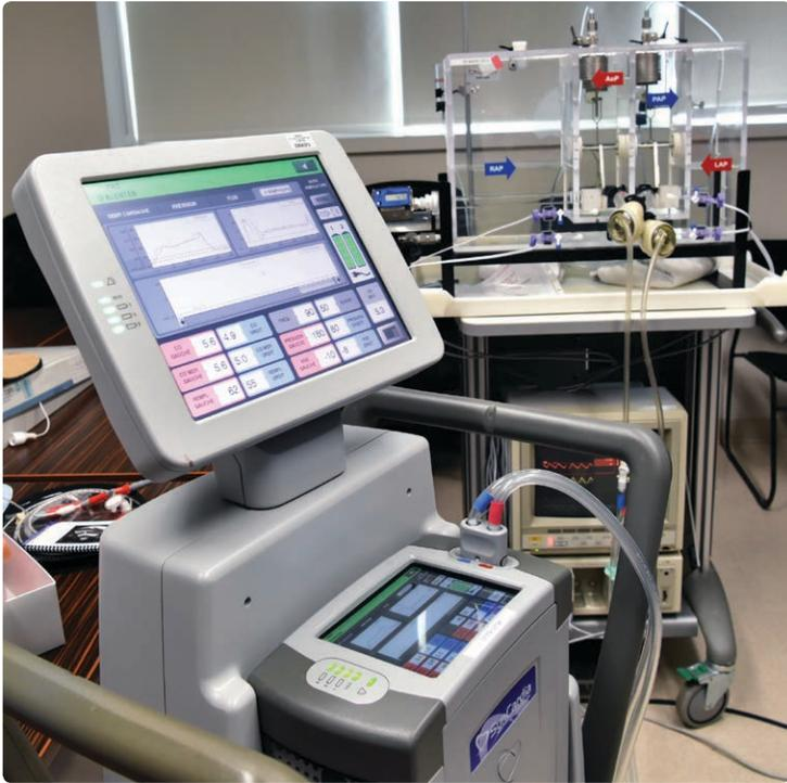
**The Syncardia total temporary artificial heart** is a blood pump that can be implanted in patients' chests suffering from biventricular cardiac insufficiency. The artificial heart is composed of two artificial ventricles which temporarily replace defective ventricles until a heart transplant is possible. It is supplied by the blood from the circulatory system and pumps it to the rest of the body to ensure adequate perfusion to all organs.
